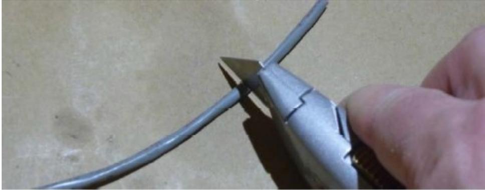
2. Use a utility knife with a new, sharp blade to cut the plastic jacket of the shielded cable 3/4" back from the end. Hold the blade perpendicular to the cable, and draw it across the cable lightly as you rotate the cable along its long dimension. This creates a scored line through the plastic jacket. With a sharp blade, not much pressure is needed. You may need a bit of practice to get the feel.
