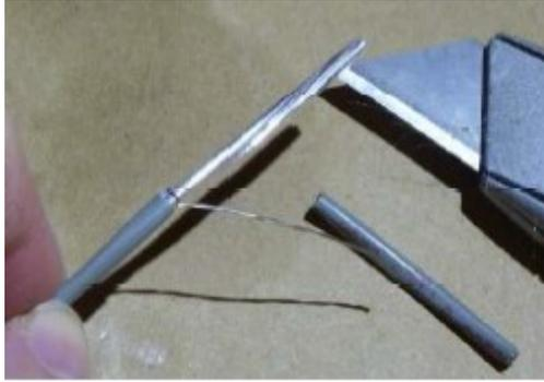
5. Separate and twist the drain wire.
