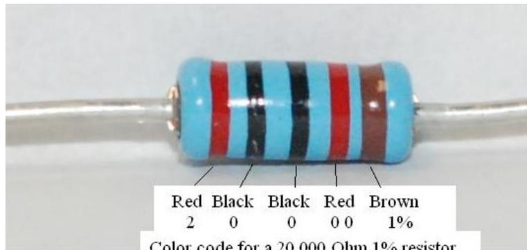
**Figure 20-demonstrating the resistor color code**
