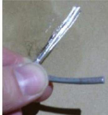
3. If you've scored the jacket carefully, you can separate the jacket at the score line without using tools. Pull the insulating jacket off, exposing the cable, showing the foil shield, the drain wire, and the fuzzy string. The result is shown here, with the foil shield showing.
