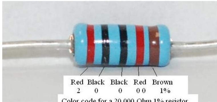
**Figure 20-demonstrating the resistor color code**
